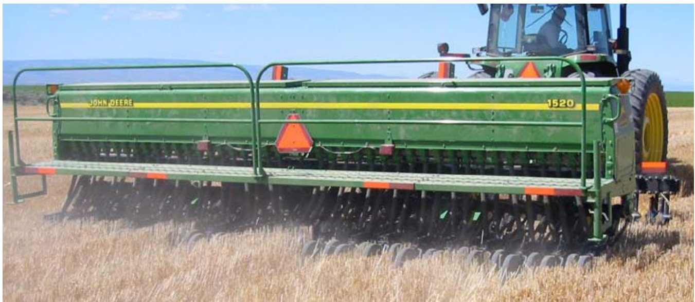
Figure 19. No-till drill planting a cover crop into wheat stubble. (Photo: McGuire)
