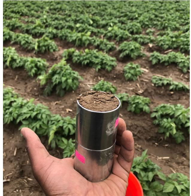
Figure 23. Researchers taking soil bulk density samples to evaluate soil health in Columbia Basin potato fields. (Photo: Sarpong)
