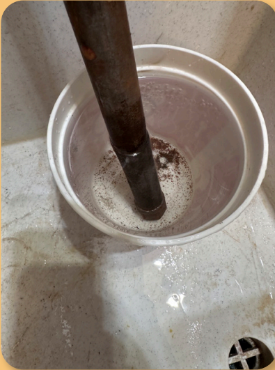
Soaking a rusted soil probe in a container with white vinegar.
