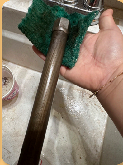
Scrubbing away rust with a heavy-duty scouring pad.
