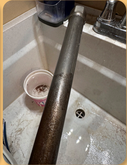
Rust-free top end of the probe with uncleaned, rusty middle portion for comparison.
