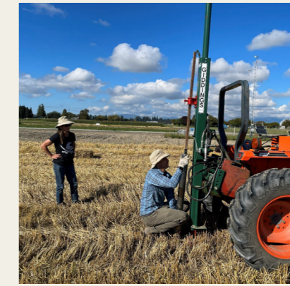
Liz Myhre, Agricultural Research Technologist, and Gabe LaHue, Associate Professor of Soil Science, using a hydraulic probe to take deep soil cores to measure soil bulk density and ultimately, soil carbon stocks. Photo by Betsy Schacht
